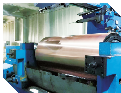
铸轧机铜辊套。张云涵 摄
